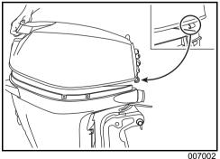
Replace the filler cap and tighten securely. Reinstall the engine cover.
