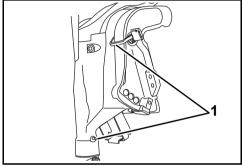
Tilt lever and swivel bracket lubrication points (annually)
