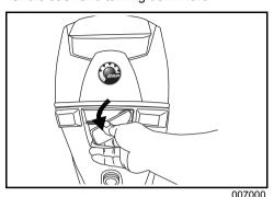
Remove the filler cap and fill the tank with the recommended outboard lubricant, as specified in Oil Requirements on page 19.
