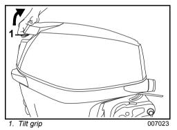
The tilt support bracket will automatically engage.
