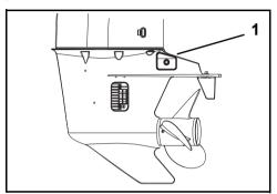
1. Anti-corrosion anode
